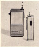
Miniature walkie-talkie has a nine-volt battery allowing communications up to three miles. Transceiver, which can be held in the palm of a hand, is 43/4" high, 21/8" wide and 11/8" deep. Price: less than \$80. Westinghouse, Pittsburgh.
