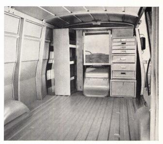
Route delivery and service installation. Plenty of space for large items, convenient bins and drawers for parts and tools.
