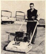
Vibro plate is designed for heavy duty soil compaction in confined areas. Model has 9,600-sq.-ft.-per-hour capacity with 5,500 lbs. of impact at speeds to 80 ft. per minute. Power is by an 8 hp gasoline engine. Wacker, Hartford, Wis.
