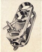
Combination jig for locksets may be used for 2\%", 2\%" or 5" backset installation. Jig is adjustable for door thicknesses from 1 5/16" to 2\%". Either hand brace or power tools can be used with the jig. Kwikset, Anaheim, Calif.
