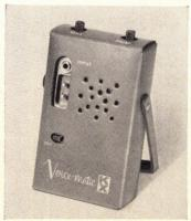
**Tape-recorder operator** is activated by the sound of a voice. Unit starts recorder when someone is talking and stops it when there is silence. A pause adjustment is included. Cost: \$34.95 with leatherette case. Kinematix, Chicago.
