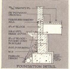
**MODULAR FOUNDATION** is steel I beams 4' o.c. bearing on second-from-top course of block.
