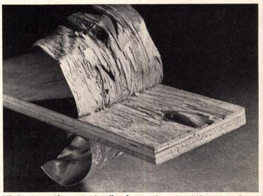
**High-strength contact adhesive** produces bonds between a large variety of core and facing materials. The reinforced elastomer is exceptionally strong as illustrated by the torn plywood above. Swift & Co., Chicago. (Circle 216 on Reader Service card)
