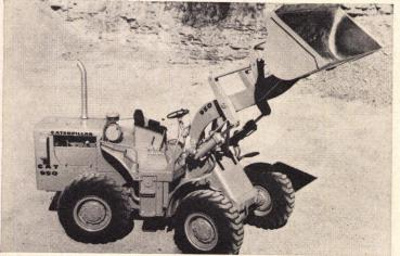
**Wheel loader** has articulated steering that can turn 35° to either side and swings the full 70° in 2.5 seconds. The 22,500-lb. loader has dual brakes for each axle, a static tipping load rating of 16,750 lbs. straight ahead and 15,250 lbs. in full turn. Caterpillar, Peoria.
