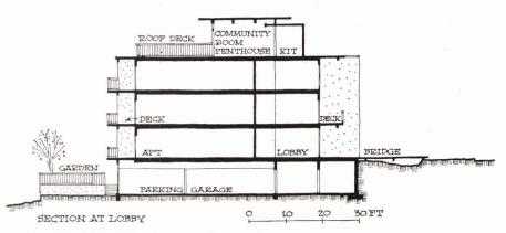
**SECTION DRAWING** shows penthouse, three apartment levels and garage set into hillside.
