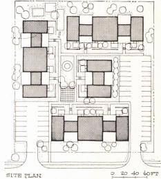
SITE PLAN shows patio bridges between pairs of buildings. Parking is kept at sides of site.
