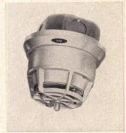
Fire protection device detects smoke and combustion gasses before flame starts. Unit fits flush with ceiling and works on 110 volts. Pilot light assures proper functioning and shows location of danger when alarm is sounded. BRK, Skokie, Ill.
