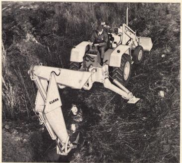
Backhoe-loader is an integrally designed unit with a single full-swivel seat from which driver can control all operations. Clark 700 has an 18' 6" backhoe reach and an 80"-wide bucket loader. Clark Equipment Co., Battle Creek, Mich. (Circle 228 on Reader Service card)
