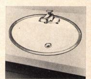
**China lavatory** for countertops has a fittings ledge designed into the 19" x 17" oval. Advantages of the integral ledge, according to the manufacturer, are narrower countertops and drainage into the basin. American-Standard, New York City.
