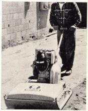
**Soil compactor** handles up to 6,500 sq. ft. of compaction per hour. It compacts layers of soil up to 28" deep at one pass and travels up to 60 ft. per minute. Model VPD 880 is powered by an air cooled diesel engine, Wacker Corp., Hartford, Wis.
