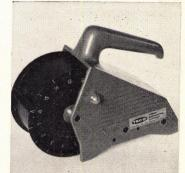
Framing marker has a marking wheel designed to place a mark every 16". Mark 16 has an automatic inking roller and can be used to mark wood, steel or concrete. Additional inserts can be used for 8", 12" and 24" spacings. TECO, Washington, D.C.
