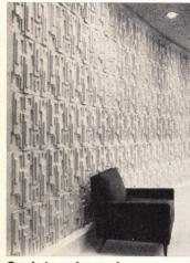
**Sculptured panels** are precast and come in four finishes: natural gray, smooth and etched white and buff. Wall-facing units weigh 35 lbs. and are 15<sup>3</sup>/<sub>4</sub>" square with a basic thickness of 1½". Nitterhouse Concrete Prods., Chambersburg, Pa.
