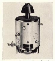
has copper tank and high gas input. At 100° rise it will supply 168 gals. per hour continuously. Thermostat is adjustable from 120° to 180°. A valve for two-temperature hot water service is available. Ruud Mfg., Chicago. Circle 331 on Reader Service card
