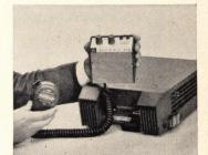
Mobile radio uses UHF channels since VHF channels are congested in most areas. Accent 450-UHF unit has the speaker built into the control head. It plugs into the radio unit for dashboard or trunk installation. General Electric, Lynchburg, Va. Circle 323 on Reader Service card
