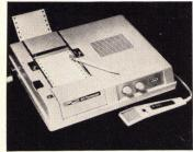
**Dictating machine** has 3"-wide tape 50' long with exposed writing surface for notes on one side and magnetic recording media on the back. Tape moves about 3" a minute and records about three hours a tape. Ansafone, Inglewood, Calif.
