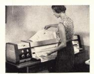
Whiteprinter has servo-motor generator drive that gives continuous speed adjustment, reversability and constant torque. Blu-Ray Model 842 is a 42" combination printer-developer that produces diazo copies for 1¢ a sq. ft. Blu-Ray, Essex, Conn.
