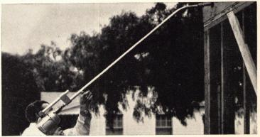
Extension drill is 60" long to facilitate drilling joists from the floor below. It can handle 4" holes in wood and 1" holes in masonry and fits all ½" drills. It weighs 6½ lbs. and lists for \$54.40. Price & Rutzebeck, Hayward, Calif. (Circle 319 on Reader Service card)
