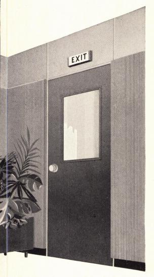
New Imperial Doors are available now in two models — the "Windsor" Series 638,  $1\frac{3}{8}$ " thick, and the "Barclay" Series 634,  $1\frac{3}{4}$ " thick. Both feature full flush design, easily adaptable to any glass or louver treatment, integral hinge reinforcement, integral lock reinforcement, and integral fully welded perimeter channel.
