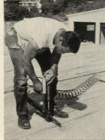
Utility nailer will drive up to 120 nails per minute in sizes up to 8d. Air-driven Powersert unit is fed by cartridges of 50 nails stitched together. Special purpose nails can be used. United Shoe Machinery, Boston.
