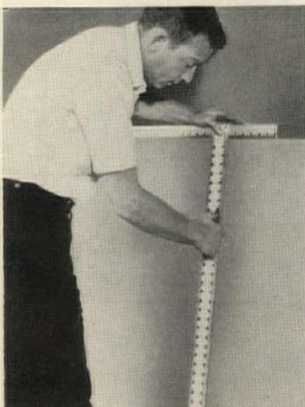
Drywall T-square has holes at 16", 24" and 32" readings for fast marking of stud lines. Short end is 22½" long, long end is 48" to span the full width of a drywall panel. Goldblatt Tool Co., Kansas City, Mo.
