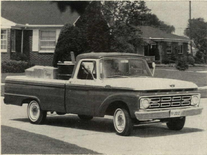
Light-duty truck , the F-100, has a straight-line bed (no rear wheel jogs) and a new heavy-duty tailgate operated by a one-hand latch. Wheelbase is 128"—6" longer than previous models; brakes are self-adjusting. Ford, Dearborn, Mich. (For details, check No. 80 on p. 209)
