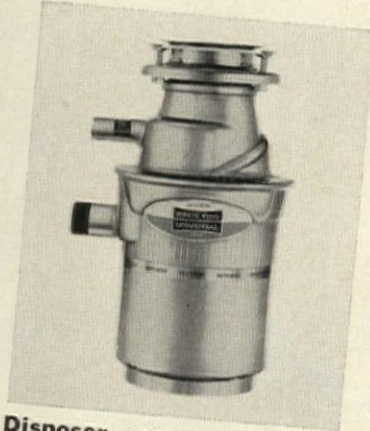
Disposer cuts vibration noise because a rubber mount suspends it free of the sink. The drain pipe connection also absorbs vibrations. Hush 3,000 has a swivel-mounted impeller to prevent jamming. Waste King, Los Angeles.
