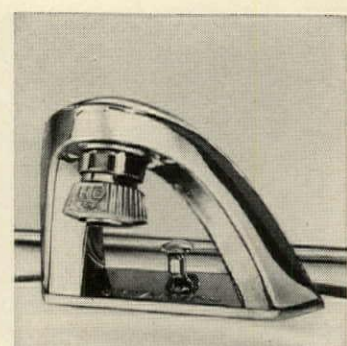
Lavatory fixture , the Cobra-Centerset, has combined spigot and control handle mounted out over the basin so water can be controlled without dripping soap on the back rim of the basin. Graning, Los Angeles. For details, check No. 19 on p. 209
