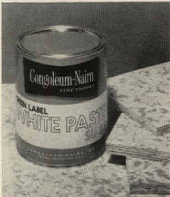
Light-colored adhesive is a white paste that can be used under translucent vinyl instead of costlier latex adhesive. SU-23 should not be used in damp places or on impervious surfaces. Congoleum-Nairn, Kearny, N.J.
