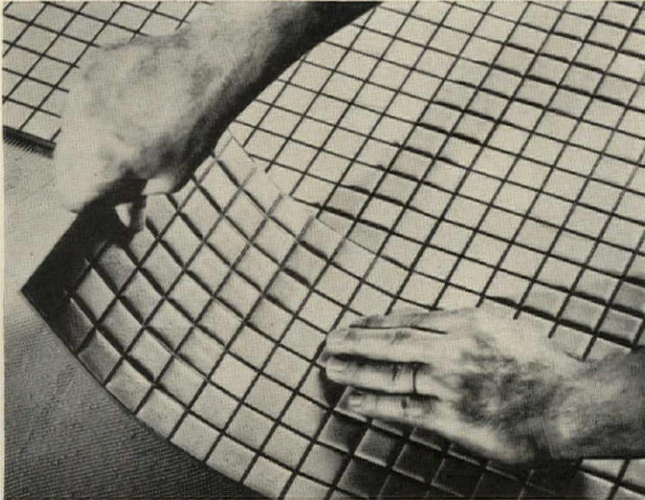
Resilient tile flooring comes in 9" sections of 1" ceramic tiles in a rubber grid. Grid is light grey; tiles are white with accents in six colors and nine patterns. Sections are set in adhesive. Grid eliminates grouting. U.S. Ceramic Tile, Cleveland. (Check No. 71 on p. 209)
