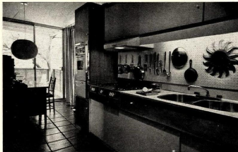
KITCHEN AND BREAKFAST ROOM of two-bedroom unit open to sundeck. Floors are Mexican tile. Interior walls have Philippine mahogany paneling.
