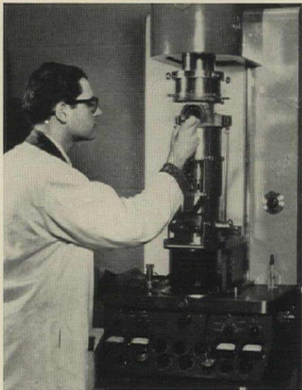
ELECTRON MICROSCOPE in Physics Lab checks surface and structure of glass fiber.
