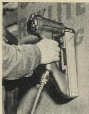
Air-driven DUO-FAST Staple Nailer makes short work of sheathing job.
