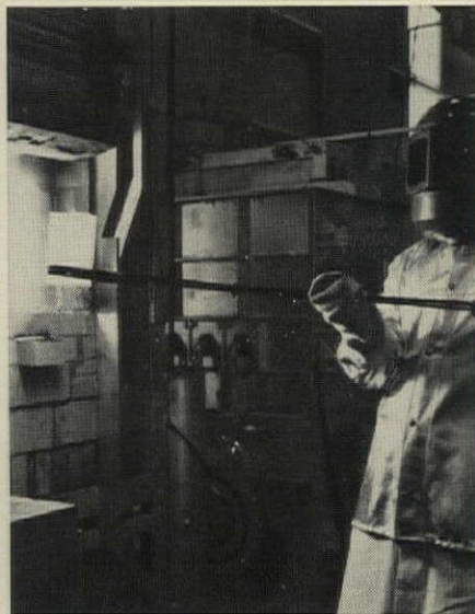
FURNACE in Mechanical Lab, used to develop new types of glass, reaches 2,600F.
