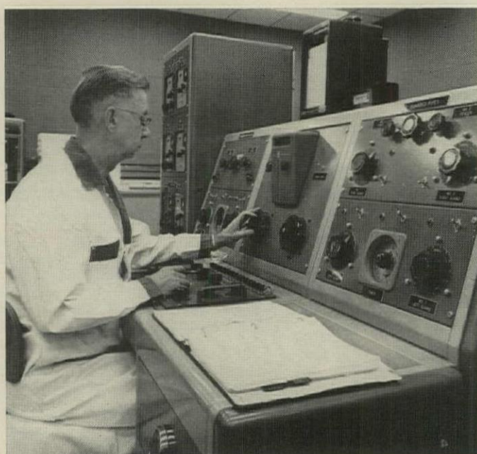
CONTROL CONSOLE in Product Testing Lab lets operator adjust temperatures, then measures and records thermal coefficients of insulation.
