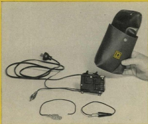
ABOVE • No bag of tricks—a QO breaker, a lamp cord, a receptacle, a few spring clips and a paper clip are all it takes to prove QO's case by actual performance.
