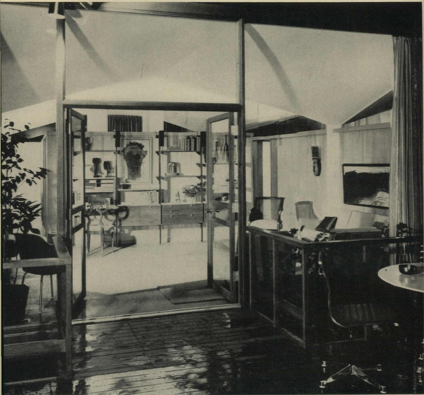
LIVING ROOM is separated from deck in foreground only by glass and slim mullions. White post at right is one of four main columns.
