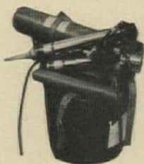
GUN for applying sealer to wall seams.
