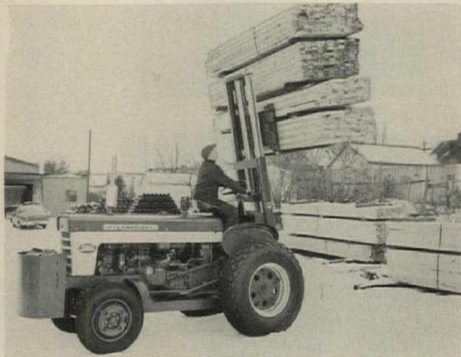
DIG LUMBER LOAD —here about 4,000 bd ft—can be moved about yard, plant, or site at 10 mph. Trucks will lift and carry up to 3 tons.
