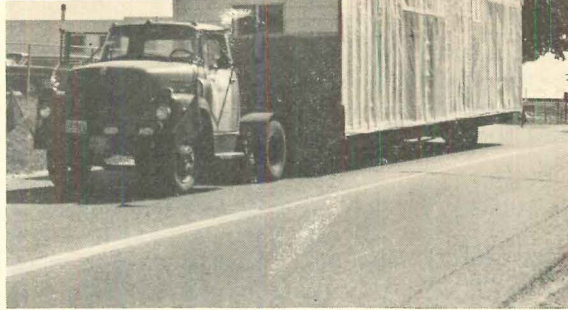
ON ROAD each unit of two-section house is trucked to site. Sections are 48' long, 9'10" wide.
