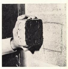
New epoxy glue from Permacel is specially designed for adhering junction boxes to concrete or masonry walls. The two-part adhesive will tack a box in place in less than two minutes. After the resin is mixed, it has a pot life of 30 minutes; at 70F it will cure to full strength in three to four hours. Cured bond is stronger than the wall itself.
