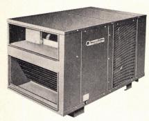
The American-Standard Packaged Heat Pump, consists of an outdoor unit and an indoor unit in just one jacket. It is usually installed through an outside wall of the home so that half the unit is inside the home, half outside—or the entire unit may be put outside and connected through the wall with ductwork. The unit provides the most compact and inexpensive type of year-round air conditioning possible.
