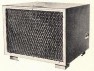
The American-Standard Split System Heat Pump consists of two units—an indoor unit with a heating and cooling coil plus an air distribution blower, and an outdoor unit consisting of the refrigerant compressor, fan and a second heating-cooling coil. The indoor unit is located at any convenient place in the ductwork. It is connected by refrigerant tubing to the outside unit, located any convenient place outdoors.
