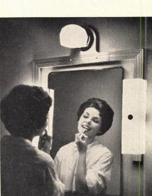
Side lighting for bathroom mirrors is provided by Dondelco's 3-D lighting fixture. Adjustable side arms have inside dimension of 19" to 23"; 5" of clear wall is needed on each side of cabinet. In remodeling uses, fixture ties into centermounted top light mounted 1" to 6" over mirror. Sidelights take two 60-w bulbs.
