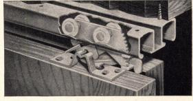
NEW SERIES 600 FA KENNATRACK... for quick, simple installation of 1" to 1¾" By-passing Doors. Kennatrack's exclusive top mount hanger eliminates extra millwork, permits maximum adjustment as well as instant removal and replacement of door without disturbing adjustment. Two hangers per door with eight floating wheels attached to grease-grooved axles that automatically compensate for door warpage. For doors up to 100 lbs.
