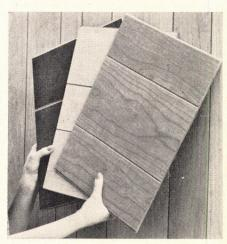
Cherry-grained hardboard is made by Celotex in three tones—imperial, blond, and bleached (above, 1 to r)—in 16" x 8' and 2' x 8' panels for use with Handi-Clip and Handi-Wall systems respectively. The panels also come in three designs—plain, regular grooved, and random grooved.
