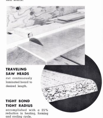
doors; furniture, and wall panels; and as complete cabinet wrapping. Solvent-type, contact-bonding adhesives offer the greatest advantages in production and forming, but other types of adhesives can be used successfully.
