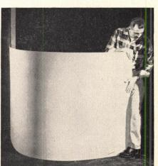
Flexible asbestos cement can be bent into a circle of 18" diameter and can be nailed or stapled ½" from its edge. The 4'x8' sheets come ½", 3/16", or ½" thick. Kamwall is proof against fire, rot, vermin, water. It is workable with carpenter tools
