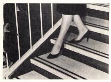
**Safety stair treads** have two 1" abrasive friction strips built into the leading edge. They also have an added 1/16" thickness of rubber wear surface in the first 4" of step area. New tread comes in four lengths—36", 48", 66", and 72"—and in 27 colors to match company's floor tile and core base designs.
