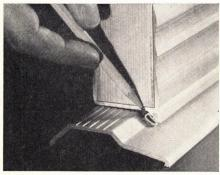
Weather and insect seal is provided by a new aluminum threshold and scuff plate. The threshold has no toe- or heelcatching edges and no dirt-catching undercuts. The scuff guard can be installed on either side of door, has full-width vinyl tube to form tight pressure seal. Finish is mill, polished, satin, or gold anodized.
