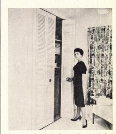
Louvered steel doors for wardrobes and closets make full width accesssible. Louvered top panel allows free air circulation, and the solid bottom panel keeps out dust. Doors come 3', 4', 5', or 6' wide, 6'8" or 8' high. Antique ivory finish can serve as neutral primer. Nylon pivots, brass pulls, upper and lower track, and all hardware are supplied.
