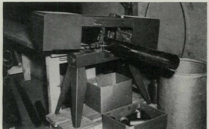
BAND SAW makes 75 to 100 cuts an hour on drain tubing—is 15 times faster than conventional hand cutting. Tubing (3" or 4") rests on bench (behind saw); cut-off pieces drop into box in foreground. National says use of band saw assures square cuts, which make for tight joints when lengths of tubing are assembled.
