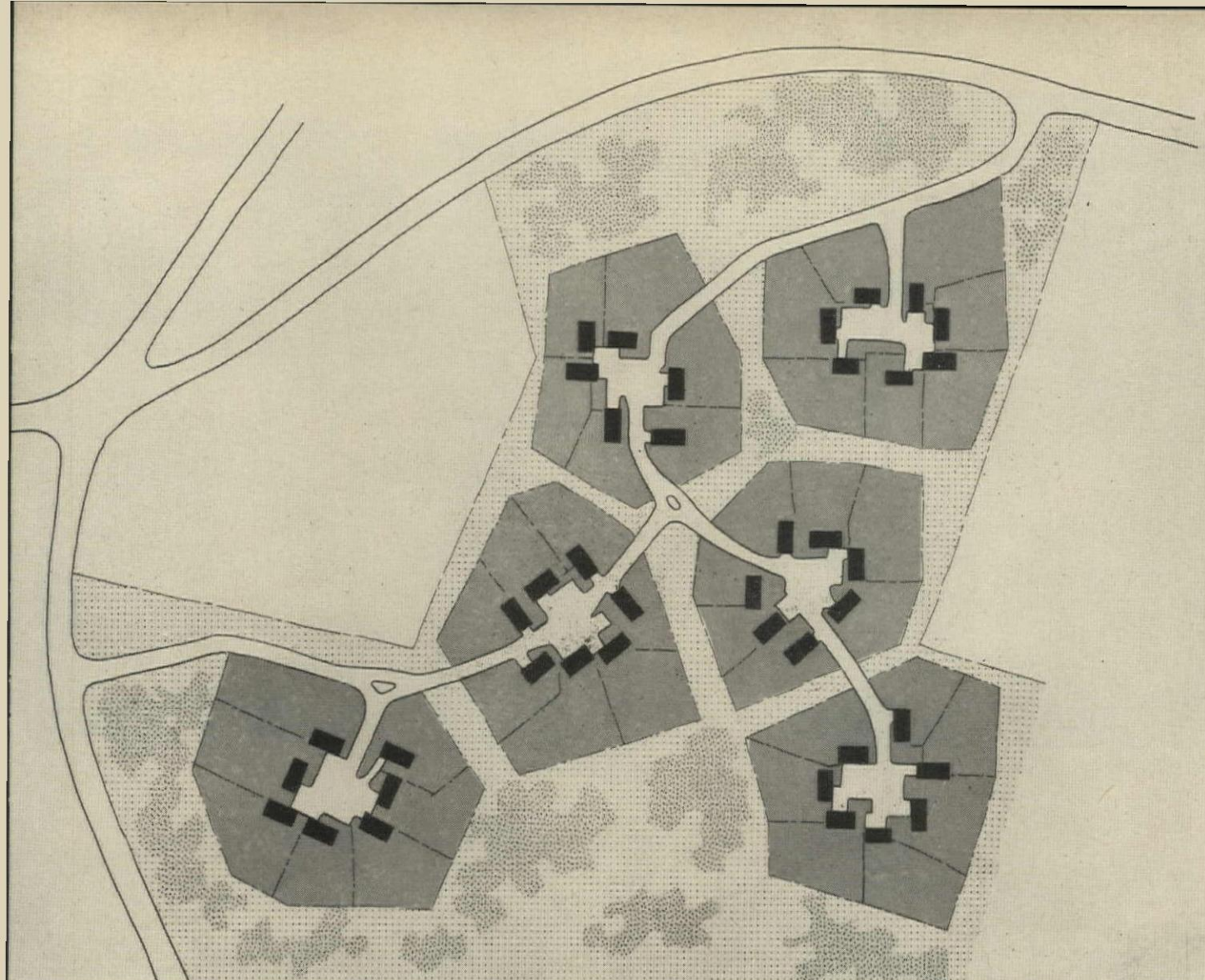
ST LOUIS CLUSTER LAYOUT in one-acre zoning area, has roads through center of each cluster. Architect Roger Montgomery, designer.
