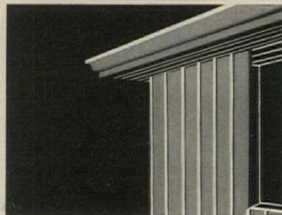
Gutter, Fascia, Board and Batten Siding
