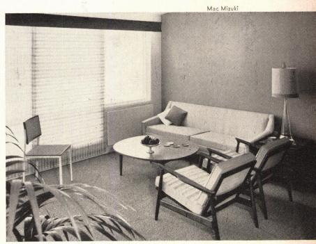
INSIDE BAFFLE covers inner face of heat pump—in far corner under window—and blends with walls, windows and furnishings.
