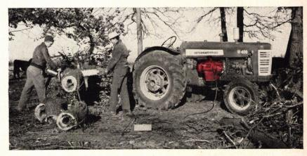
Now! "central station" electric power on wheels! The International W 450 may be equipped with Electrall®, mounted as shown in red. Electrall powers any equipment normally operated from a 5 to 71/2 kva high-line transformer. Trailing Electrall can be pto-operated by any tractor of 30 hp or larger.
