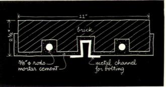
**SECTION OF PANEL** shows how channel and deformed-rod reinforcing is cast into the panels. Except for the three slots, brick is standard 2½" x 11" Norman. Almost any brick face could be used, including 12" x 12" Roman. Cement backing takes up variation in brick thickness. Machines to make panels will cost brickyards at least \$20,000.
