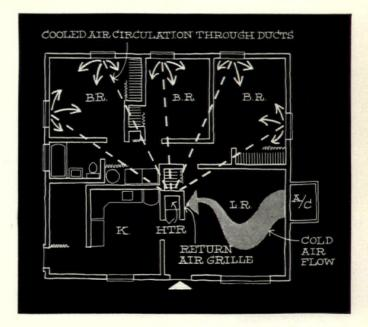
grill. The furnace fan drives the cool air through the heating ducts (dotted arrow) to whatever rooms the owner wishes to cool. At night, for example, the home owner can close the register in the kitchen, send all the cool air to the bedrooms, as shown here. The living room gets the cool air first, is obviously cooled more than the other rooms.
