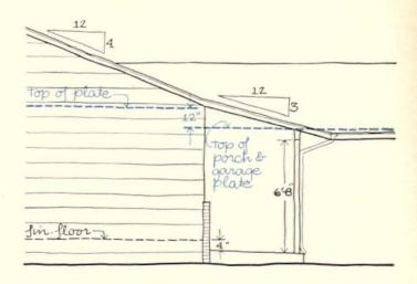
**THE PORCH** is mostly for looks (see Reason No. 3). This detail shows how it brings the eave line down and the base line up. The porch floor slopes 1" away from the house, and the front yard is graded up. Note low ridge of garage 100f.
