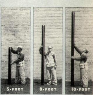
PERMALINE PIPE comes in 5-foot lengths in 2", 4", 6", and 8" sizes; 8-foot in 3", 4", and 5"; 10-foot lengths in 4" and 6".
