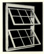
f. Wood awning window gets a Colonial look with panes sectioned into six or eight lights. Window uses same operating mechanism as Woodco E-Zee Loc standard model, offers easy operation, sturdy locking mechanism, concealed hardware, double-vinyl weatherstripping, and easy cleaning. Window comes in about 175 sizes for stud openings from 22" x 20½" up to 153¾" x 52¾" for multiple window arrangements. Prices vary according to arrangement. Woodco Corp., North Bergen, N. J.
