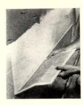
g. Ceramic Suntile now comes in 12-tile sheets for quick installation. 41/4" sq. tiles are mounted on a specially developed mesh of treated, glossy jute. Mesh-backed sheet is bonded to wall with adhesive, self-curing mortar or regular portland cement mortar with a bonding coat of self-curing mortar. Tiles are spaced for grouting and do not require soaking. You can get the new "Setfast" sheets in Suntile's 16 most popular glazes. Cambridge Tile Mfg. Co., Cincinnati.
