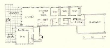
**FLOOR PLAN** shows the large amount of window area made possible by the strength of the structure. Interior partitions carry no load.
