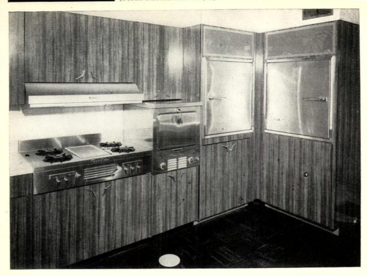
**A.** These plastic-faced cabinets and work surfaces look like fine wood. But they are made of melamine and phenolic laminates bonded to both sides of a ½" thick, 4' x 10' core with urea-formaldehyde resin. Sandwich is placed in a press, subjected to heat under pressure for bonding and curing. Warpage is impossible, maker says.
