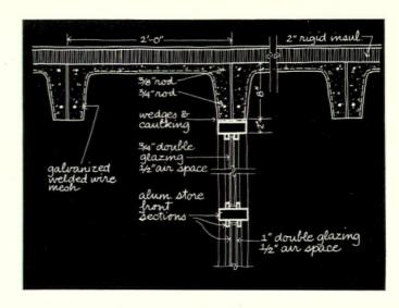
concrete Roof Channel slabs (left and above) serve as both roof deck and ceiling. Cast of reinforced lightweight expanded aggregate, they weigh only 100 lbs. per cu. ft. (vs. 150 for ordinary concrete), have good insulating value. Metal forms in which they are cast leave underside so smooth that two coats of paint finish the ceiling.
