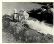
Carryable Diaphragm Pump . . . This self-priming, 120 pound diaphragm pump will handle water in the thickest sand, muck, or mud. Capacity: 5,000 g.p.h. Size: 3". Complete line of centrifugal pumps are also available in sizes from 1½" to 3".
