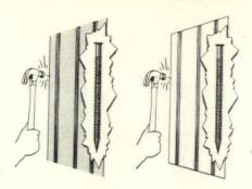
d. Stronghold annular-thread nail was made specifically for interior hardboards used on wall or ceiling applications. Nail is made of high carbon steel, heat treated and tempered. Tiny nail head is said to give a firm bearing and to be almost invisible when driven flush. 1" x .058 No. 43 nail, approximately 1298 pieces per lb., costs \$37.50 per cwt. Minimum order 50 lbs. For ivory coloring, add \$4 per cwt. Independent Nail & Packing Co., Bridgewater, Mass.
