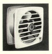
n. NuTone fan is designed for installation between rooms to "boost" air to rooms that do not completely benefit from the house's heating and cooling equipment. Thus, maker says, it provides maximum effectiveness for both heating and air conditioning systems. The fan is mounted between studding and fits a 91/4" sq. wall opening. It is adjustable for walls 25/8" to 51/4" thick, operates on standard 110-120 v. AC current. \$21.95. NuTone, Inc., Cincinnati.
