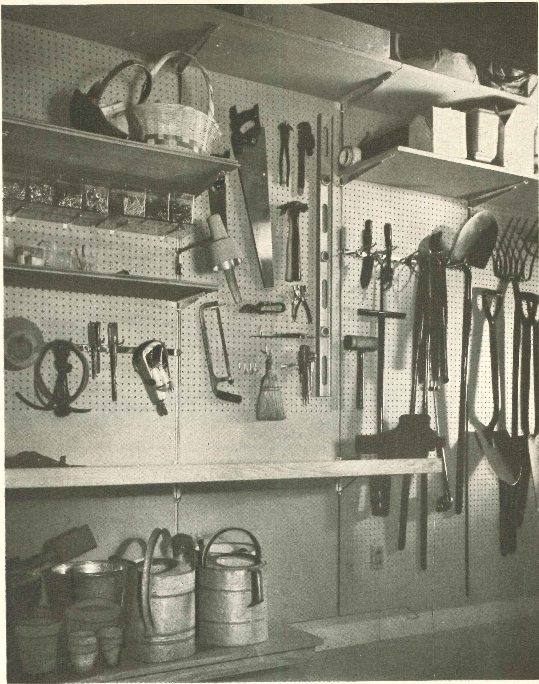
Secret of new hardware is shown above. Brackets which hold shelves are supported in vertical channel slot, cannot slip out. This hardware can carry far greater weight than perforated board. Combination of pegboard and new hardware is ideal, as shown in photograph.
