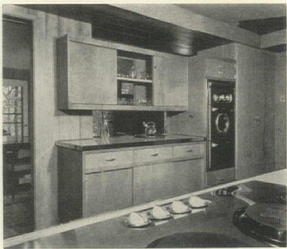
View 1 shows pass-through, built-in ovens, mahogany cabinets—features of kitchen in plush four-bedroom house built on level. Cost of one-floor plan was higher than multistories because of bigger foundations, roofs, more paneling.
