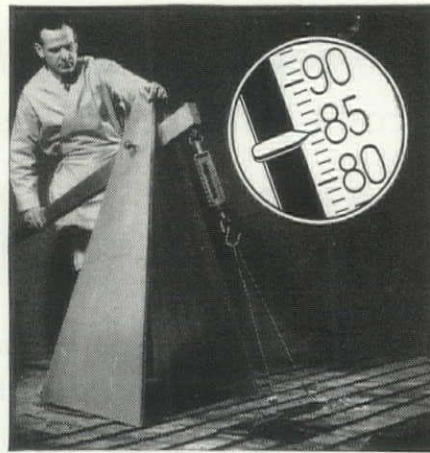
PlyScord holds nails well. Tests on roofs exposed 2 years show minimum force of 85 lbs. required to pull cedar shingle from 5/16" PlyScord. In case of asphalt shingles, roofing is invariably torn from PlyScord without loosening nails. Other tests and actual experience shows 5/16" PlyScord holds nails as well or better than 1" soft pine boards.
