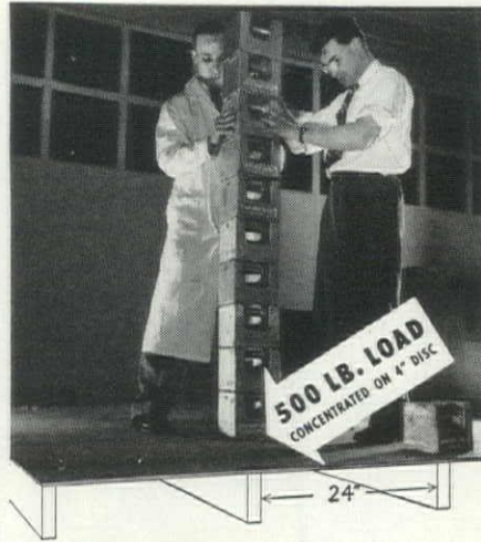
In test above 3/8" PlyScord on 24" span easily withstands 500 lb. concentrated load. Plywood's great two-way strength means economy because relatively thin panels can be used—3/8" PlyScord on rafters 24" o.c. easily withstands uniform load of 30 lbs. p.s.f., 5/16" on 16" span takes uniform load of 40 lbs. p.s.f. Both constructions now FHA accepted.
