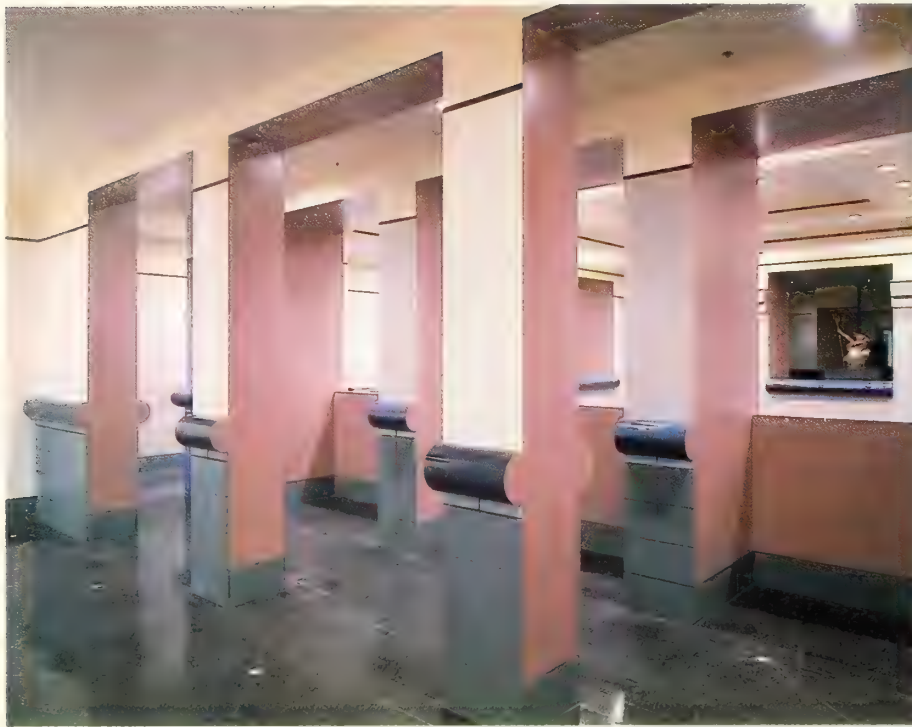
Left: Second-floor gallery surrounding the central two-story atrium. Moldings make piers seem as though they were carved from a continuous wall. Flooring is polished black terrazzo interspersed with small tiles. Framed in opening at right rear is small-scale model of Raymond Kaskey's sculpture Portlandia , an allegorical symbol of the city, to be placed over the main entrance.
