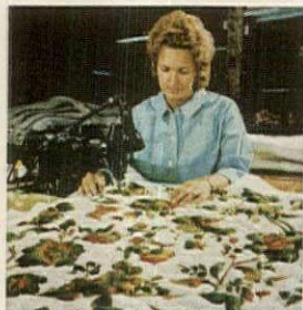
Beautiful prints are outline-quilted using lockstitch, unbreakable, continuous filament nylon thread.
