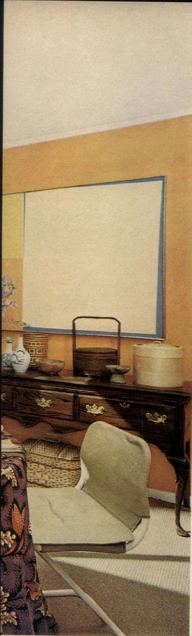
were left uncurtained. Tall plywood screens give the living room even more vertical play and can be moved across the windows if necessary. Other screens shield the front door and utility closet. A do-it-yourself idea, the screens are painted plywood panels connected with piano hinges.
