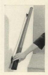
Hand railing comes in 4-, 8-, and 12-foot lengths, ready to install. Supporting brackets slide back and forth in a slot so the rail can be attached directly to the wall studs no matter where they are located. Rail swivels to match any stair pitch. Needs only a finishing coat of paint. Logan Co., 200 Cabel St., Louisville 6, Ky.
