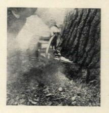
Begin tree felling with a horizontal cut low on side of trunk at right angles to direction in which you want tree to fall. To make a level cut without having saw bind or your arms drop off takes considerable practice but it is one of critical felling cuts.
