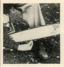
Check chain tension before each use of saw. Maker's (or rental agent's) instructions will note location of take-up adjustment for your model. A chain that is too tight may overload saw. One that is too loose may be inefficient and dangerous. Picture gives idea of proper tension.
