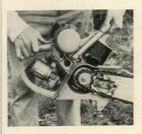
Lubricate chain and sprocket by means of plunger provided on all saws (making sure, of course, that oil supply is adequate). Frequent squirts of oil are essential to proper operation and long life of saw teeth and chain, help keep dust from gumming works.
