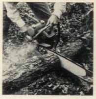
Rock saw to help teeth clear sawdust from kerf, to minimize risk of binding and, by elaboration of motion, to facilitate cutting of large-diameter logs. Be careful, however, not to twist machine while rocking it. And, above all, don't use it for leverage.
