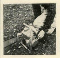
Make safe start by bracing knee against motor housing, seeing to it that saw teeth are not touching dirt or stones. Apply pull on the starting handle directly in line with direction of resistance. Otherwise, saw may whip out of hand. Keep throttle control low.
