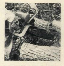
Resort to undercut when a log must be cut between points of support. But remember that when top of chain is cutting, kick-back of saw is reversed. Make sure that cut pieces will fall clear. With undercuts, pressure must be applied by lifting.
