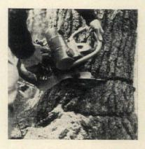
Open vital notch with second cut above first, angled downward so it will meet inner line of first cut exactly at right angles to direction of the fall. Notch should reach just short of center of the trunk. Beware lest notch piece binds before it kicks out.
