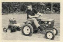
Self-Powered Tiller. A Wheel Horse attaching tool for the serious gardener. Has own  $5\frac{1}{2}$  hp. engine. Designed to dig deep through hard packed earth. Other garden tools include plow, cultivator, disc.
