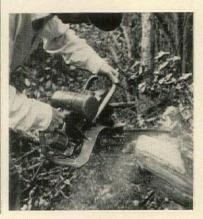
Practice lopping cut until you get used to kick of chain as teeth bite into wood. Accustom yourself to releasing the throttle the instant saw snags, binds or appears to be operating improperly. Don't bear down on this top cut; let gravity do all the work.
