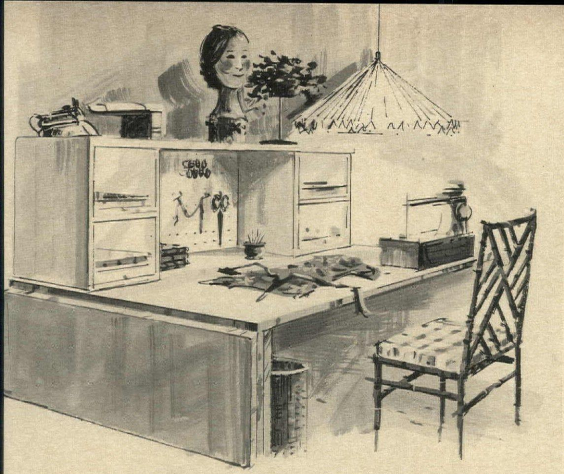
A SEWING CENTER IN THE FAMILY ROOM keeps all the tools of the trade in one spot and instantly visible. The arrangement consists of two two-drawer storage units for patterns, trimmings and other small sewing essentials, plus a 4-by-8-foot sheet of plywood. A 2-foot section of the plywood is cut off, then hinged to the larger piece to make a drop leaf, and a plywood shelf steadies drawer units on top. Perforated hardboard at back of niche makes a parking place for scissors, spools. Total price of four drawers: about $22.
