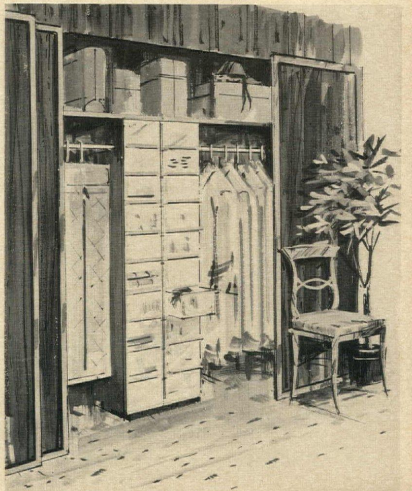
INDIVIDUAL TIERS OF STORAGE IN A DRESSING ROOM keep a husband's and wife's accessories in order without encroaching unduly on wardrobe hanging space. To build each tier, you need two five-drawer units stacked one atop the other. Outsides of units are sheathed with plywood to support clothes poles; tops are anchored to shelf. Price of twenty drawers: about $110.
