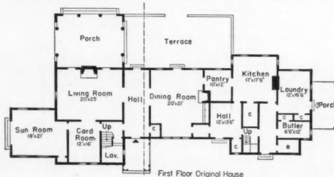
FIRST FLOOR PLAN of the old house shows the over-sized rooms, the waste hall space, the poorly laid out room arrangement. The dotted line bisecting the plan indicates where the house was cut in half by an electric saw. The north section, to the right, was moved 75 feet on a cradle and placed on a new foundation. The garage belonging to the original house was also moved and a new garage wing added to the south house.
