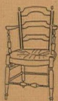
TURNED SPINDLES SUPPORT THE ARMS AND CARRY THROUGH TO THE STRETCHERS FOR ADDED SOLIDITY
