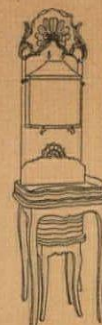
WASHBASIN OF PEWTER IN A WOOD FRAME, FROM BURGUNDY, STORAGE TANK ABOVE BASIN, SEPARATE WASTE PAIL BELOW
