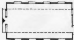
6. Simplest of all is the well-known Quonset hut. Shell only is supplied; partitions are not included. Stran-Steel.
