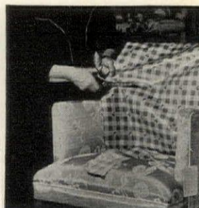
2. How to try fabric on chair once it's cut, match pattern.
