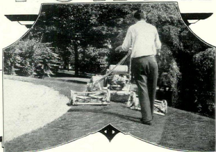
Above: Coldwell "L-Twin" Motor Lawn Mower and Roller. Mows and rolls simultaneously 4 to 6 acres a day on one gallon of gasoline. Gang units more than double its capacity.
