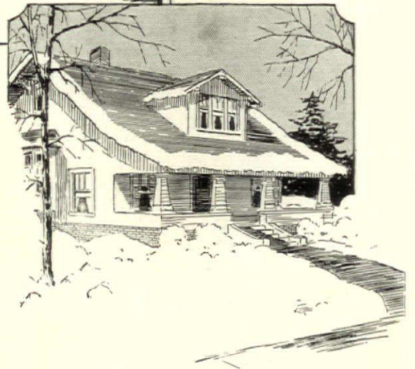
The snow covered house is warmest. Furnace heat going to waste melts the snow on the other house.
