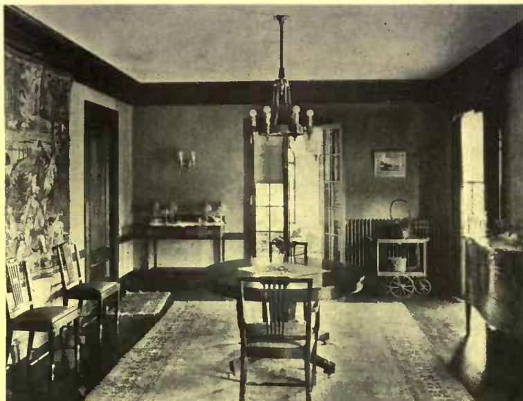
The dining-room is finished in gumwood, oiled and waxed to match Circassian walnut—a practical substitution
