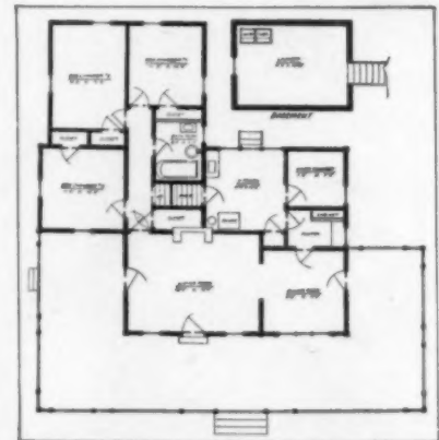
By reason of the sloping site a laundry was built under a rear corner
