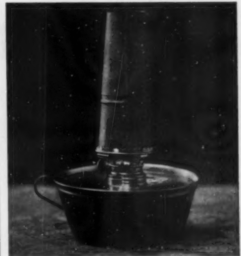
The typical incubator lamp has a metal fount with a durable handle and a metal chimney containing a mica-covered aperture opposite the flame
