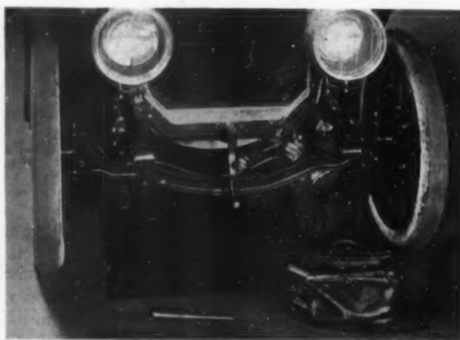
THE REPAIR PIT; TIGHTENING THE FRONT SPRING CLIP
