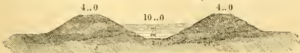
FIG. 1.—Section of Drain from O to M, and from P to R.
