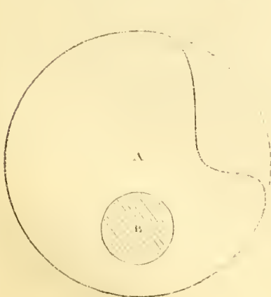
Fig. 7.—Cross Section of collapsed Boiler at h g .
