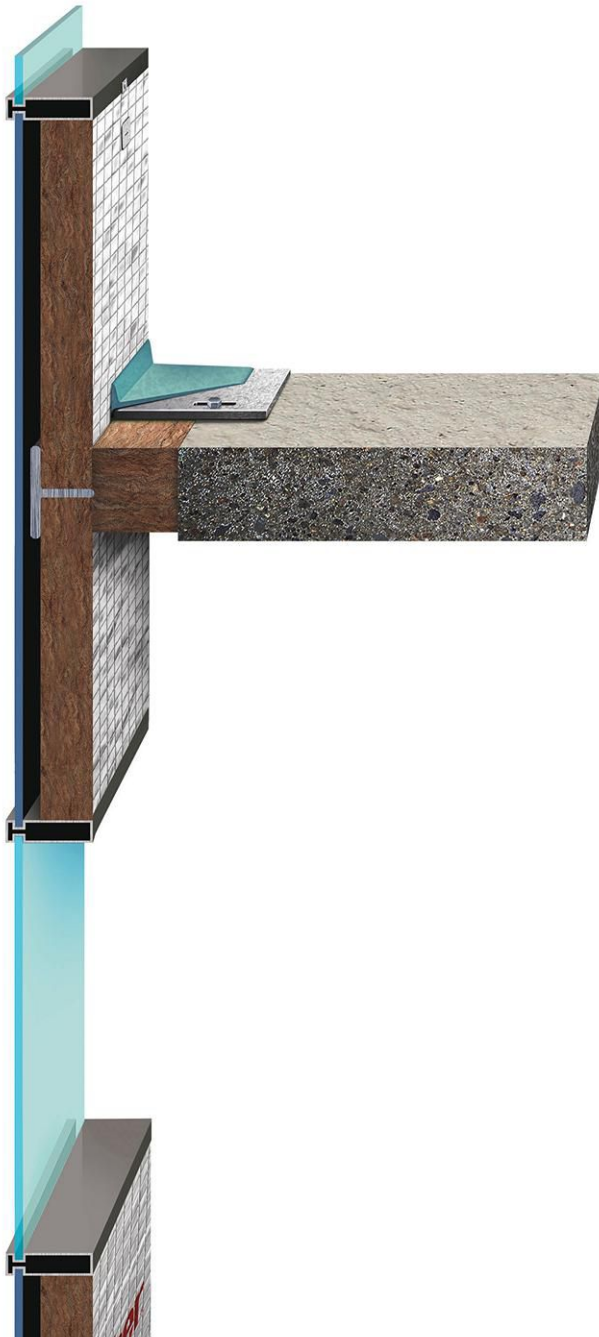
Curtain wall, joint, and floor slab
