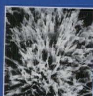
Xypex Crystallization (Mature)
