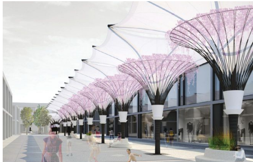
Hanging Parasol Garden combines sun shading, illumination, water collection and climbing plants into one innovative shade system.
