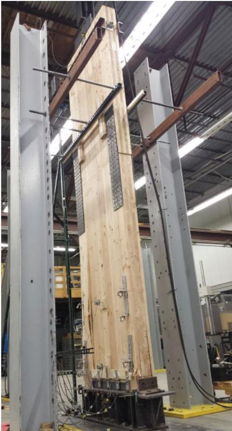
In this rocking test of a CLT shear wall, the panel maintained its lateral load-bearing strength under cycling loading to simulate seismic conditions and returned to a vertical position at completion of the test.
