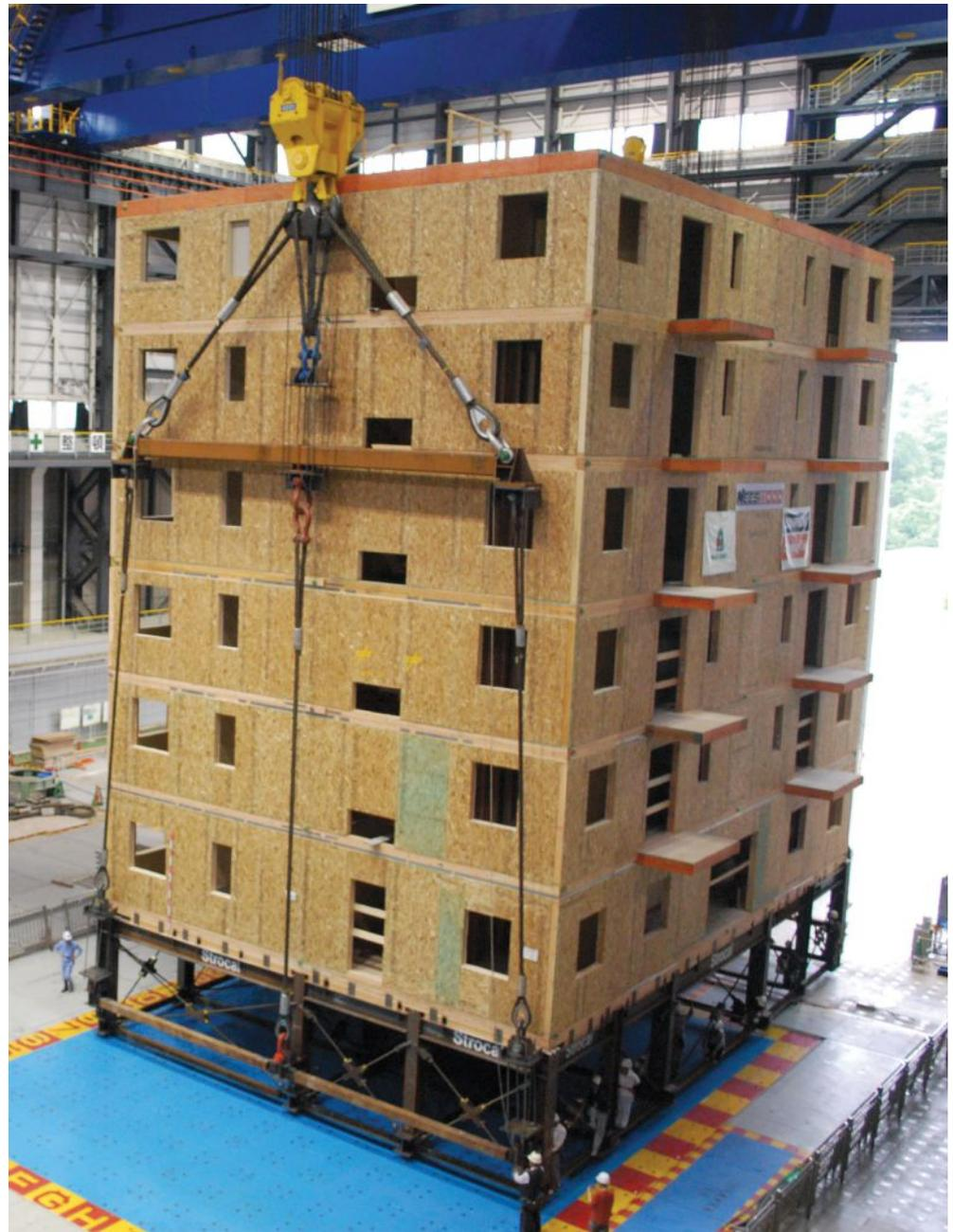
Subjected to three earthquakes on the world’s largest shake table in Miki, Japan, this full-scale wood-frame apartment building performed excellently with little damage.
