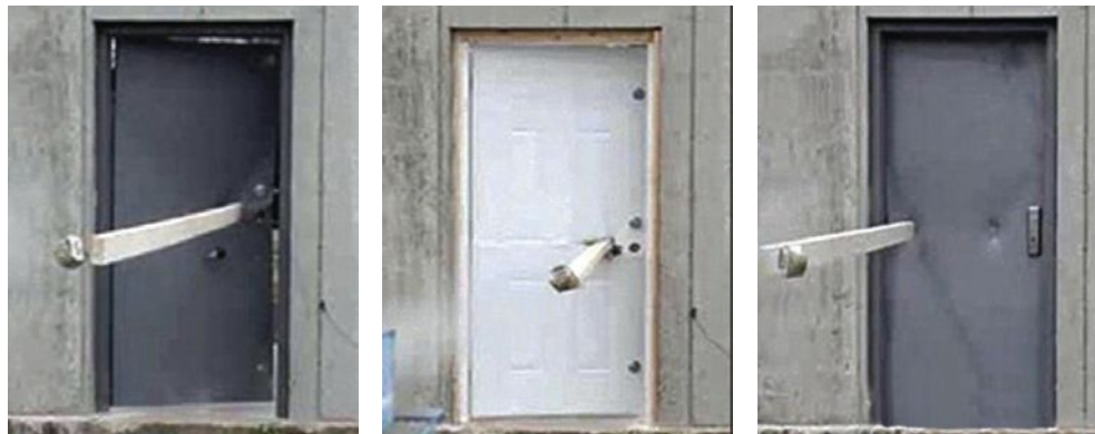
Impact test results on safe room doors show failure at the latch/lock (left), failure by full penetration (center), and a passing condition that withstood both penetration and latch/lock failure (right).
