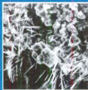
Xypex Crystallization (Initiated)
