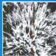
Xypex Crystallization (Mature)
