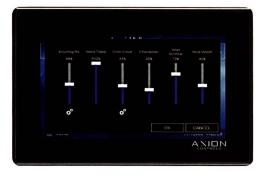
connects with mobile devices via Bluetooth, can manage up to 36 zones or can be wirelessly ganged with up to seven additional stations, to control as many as 288 zones. It can accommodate preset scenes, control movable fixtures, and manage intensity, color, and white-color temperature, among other settings. acuitybrands.com circle 214
