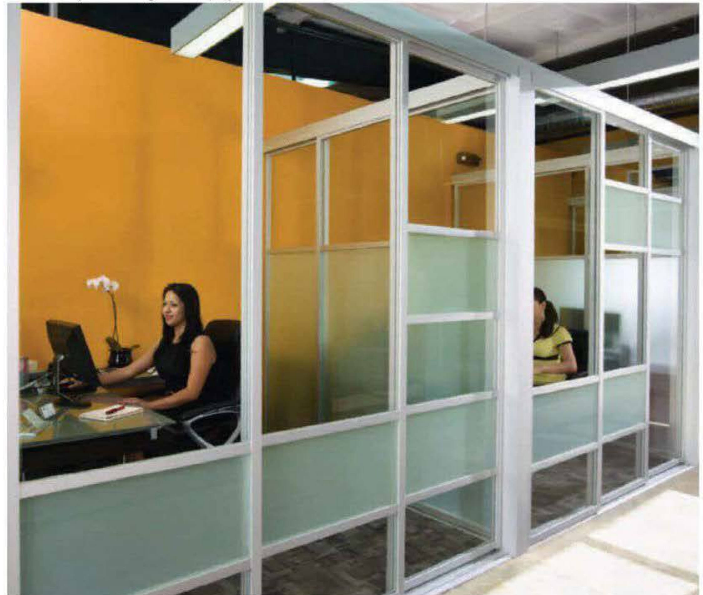
Consecutive glass partitions provide privacy and some acoustic performance while offering daylight and a sense of openness.
