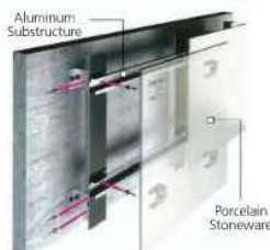
Cross-section of Marazzi's Ventilated Wall System
