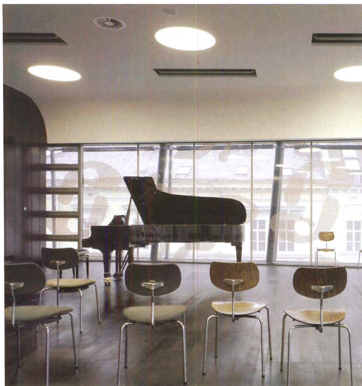
Informal recital spaces provide students at the music school with views of the surrounding neighborhood. The woven metal skin over the glass facade, which is silk-screened with stylized musical clefs, reduces solar glare.
