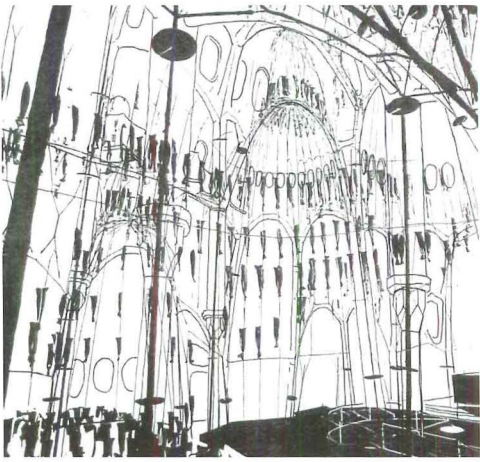
The Sagrada Família's towers are among the tallest in Barcelona (opposite). Gaudí used hanging models to determine the reversed catenary structure for the Colònia Güell chapel, incorporating his findings in the designs for the Sagrada Família (above). A drawing by
