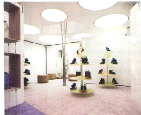
Track-mounted PAR30 halogen lamps are installed around a circular fluorescent luminaire and adjacent to the stair to highlight individual items (left and bottom). Large, round luminaires with opalescent glass diffusers illuminate the first-floor galleries (above).
