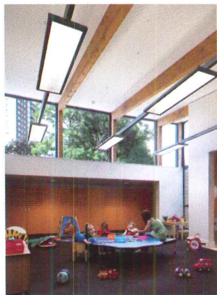
Hazelwood School's 10 classrooms feature generous storage space. Clerestory windows provide plentiful ambient daylight, without the glare, or views to the outdoors that could distract partially sighted children.
