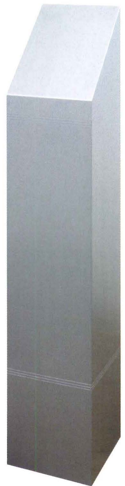
Right: Metropolitan Bollard: Square Stainless Steel or Bronze Satin Finish Size: 48" high x 8 7/8" square sides, with slanted top Custom sizes available Pipe Size: 8" Schedule 80 pipe (to be filled with concrete)
