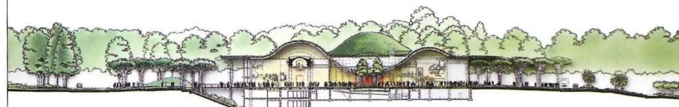
Sections through the California Academy of Sciences highlight the undulating roof and public spaces.
