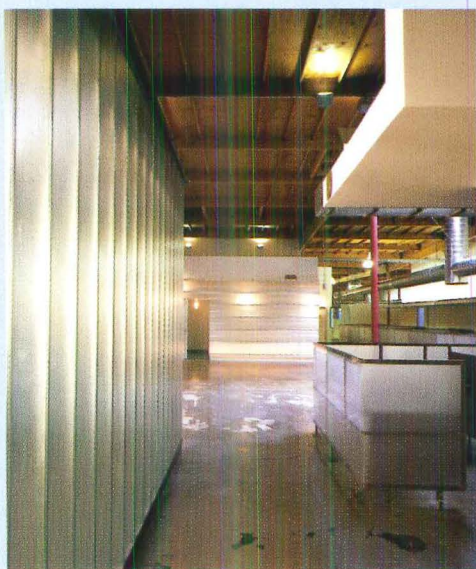
The data center at YouBet.com is enclosed by curved acrylic panels fastened to the stud wall with hat channel clips (above and far right). Workstations (right) are enclosed with single sheets of heated and bent acrylic.
