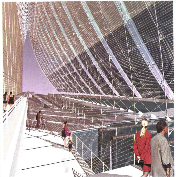
The Sun Wall competition-winning design, by Solomon Cordwell Buenz & Associates and Arup, incorporates photovoltaic panels with a solar thermal installation for hot water.
