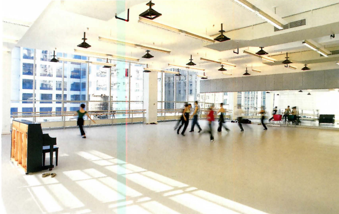
Linear indirect/direct fluorescents supplement the daylight streaming through floor-to-ceiling windows in one of 14 rehearsal studios (left). The black-box venue (below) is equipped with an array of theatrical fixtures.
